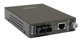
This DMC-1530SC Smart Media Converter provides intelligent functions like LLCF, LLR, store-and-forward mechanism, back-pressure, and 802.3x flow control. It converts 10/100 Mbps 10BASE-T/100BASE-TX Fast Ethernet twisted-pair signals to 100BASE-FX Fast Ethernet single-mode fiber signals. The maximum fiber cable distance is 30 km. One RJ-45 twisted-pair port and one fiber port (SC connector) are included.
