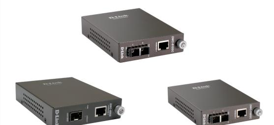
DMC-700SC Media Converter: This converter converts 1000BASE-T Gigabit twisted-pair signals to 1000BASE-SX Gigabit multi-mode fiber signals. The maximum fiber cable distance is 550 m. One RJ-45 twisted-pair port and one fiber port (SC type connector) are provided.
