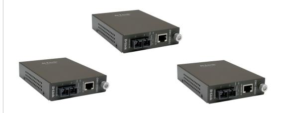
These converters convert 10/100 Mbps 10BASE-T/100BASETX Fast Ethernet twisted-pair signals to 100BASE-FX Fast Ethernet single-mode fiber signals. One RJ-45 twisted-pair port and one fiber port (SC connector) are provided.
