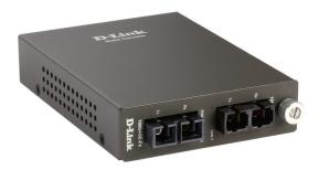
This converter converts 100BASE-FX Fast Ethernet multi-mode fiber signals to 100BASE-FX Fast Ethernet single-mode fiber signals. The maximum fiber cable distance is 15 km. Two fiber ports (SC connectors) are provided.
